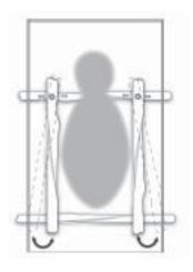
curves, particularly when shipping over long distances. The cost of construction is very cheap, using only four poles, which must be strong and resilient, and only two bolts. As for any rope used, most mahouts will have it at hand already.
